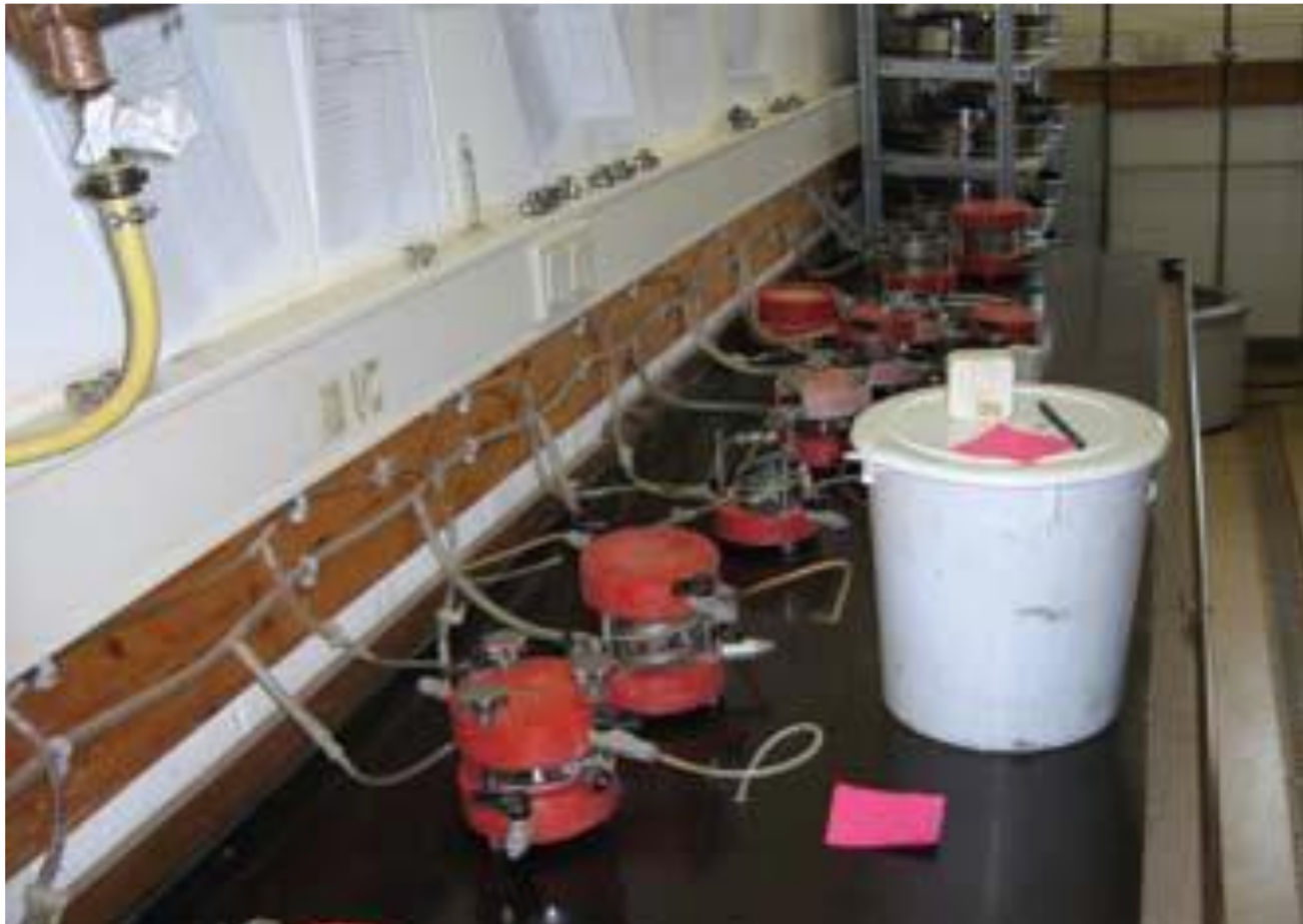
Taking the soil sample and measuring the CBR
