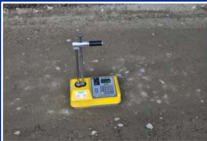
Testing on the site by using a Troxler sonde
