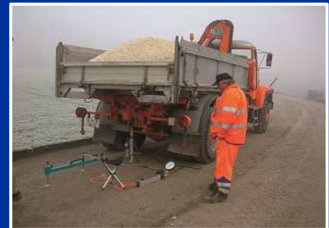
Execution of a load plate bearing test
