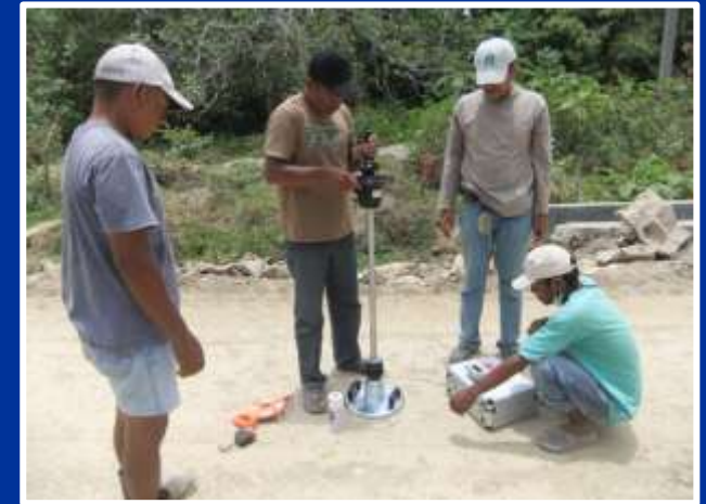
Testing on the site by using a falling weight drop tester
