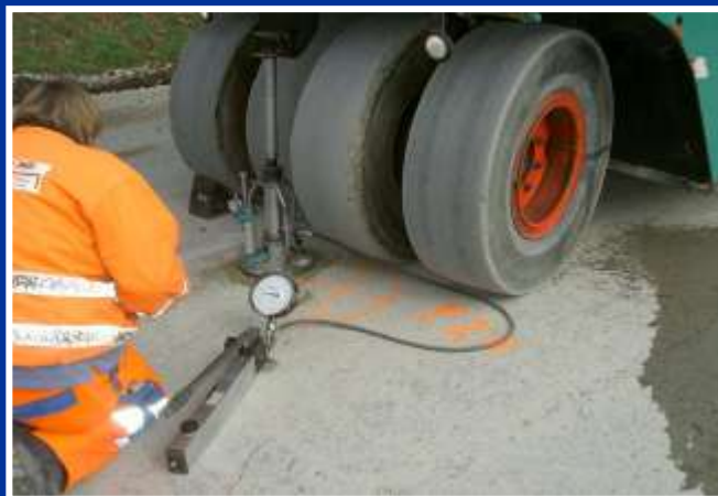
Execution of a load plate bearing test
