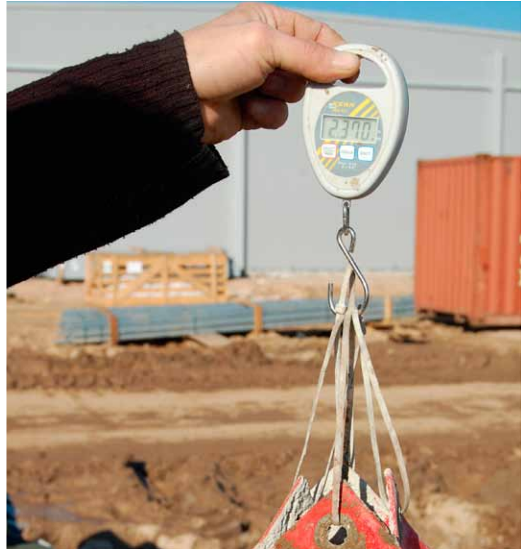
Net amount of 1,3 kg/m 2 NovoCrete® for this section (45 cm milling depth)
